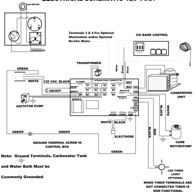
NOTE: IF USING EXTRA 120V. ACCESSORIES SUCH AS RECIRCULATING MOTOR, ILLUMINATION ETC., MAKE CONNECTIONS AT TERMINAL B3, B4 FOR POWER/BLACK LEG. TERMINALS W3, W4 FOR NEUTRAL/WHITE LEG AND GROUND AT TERMINAL G3, G4.
