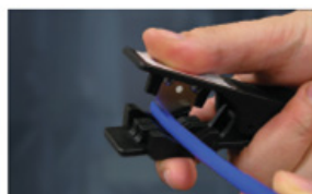
Step 1 Cut the tube square and remove any burrs or score marks. We
