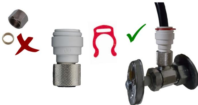
Locate the PSEI6012U9 angle stop adaptor in the UCM Install Kit. Locate the angles stop water source feeding the system, remove the compression nut and ferule ring from it and replace with the PSEI6012U9 fitting.
