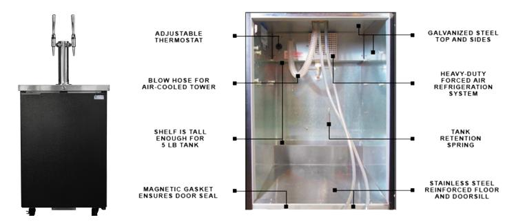
The 24" direct draw cooler is a commercial grade, heavy duty, mobile or stationary, refrigerated cabinet assembled with a two tap tower and iN2-2P Profusion unit mounted inside. The countertop is made from heavy-duty stainless steel including a built-in drip tray for easy cleaning.
