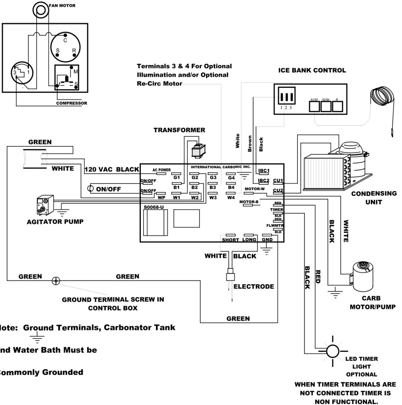
**Note: Ground Terminals, Carbonator Tank and Water Bath Must be Commonly Grounded**
