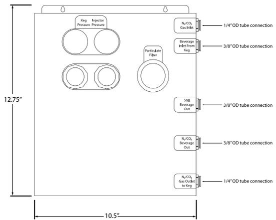
Enlarged view of iN2-2P injector
