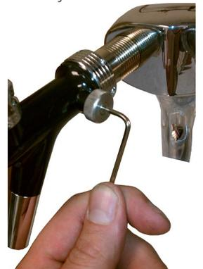
Horizontal position is full open. Downward or upward position, quarter turn restricts or slows flow from the faucet. Flow can be completely shut off if turned too far back.
