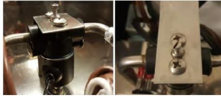
A leaking push button valve is usually caused by debris in the valve body. Follow these easy steps to clean out. Always unplug unit before working on it.
