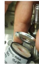
10. Before putting the solenoid back on the stem, position the washer so the groove is up, in the solenoid. Check that wires in
