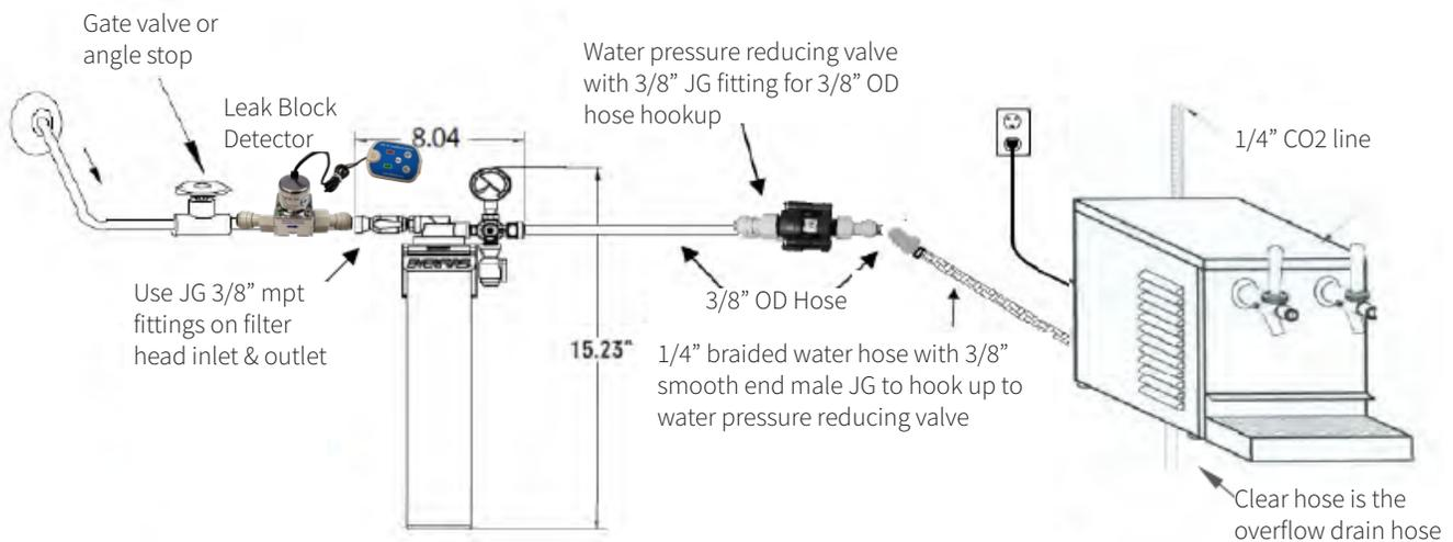
Tighten PI451214FS 1/2" to 3/8" JG fitting to inlet and outlet of water pressure reducing valve
