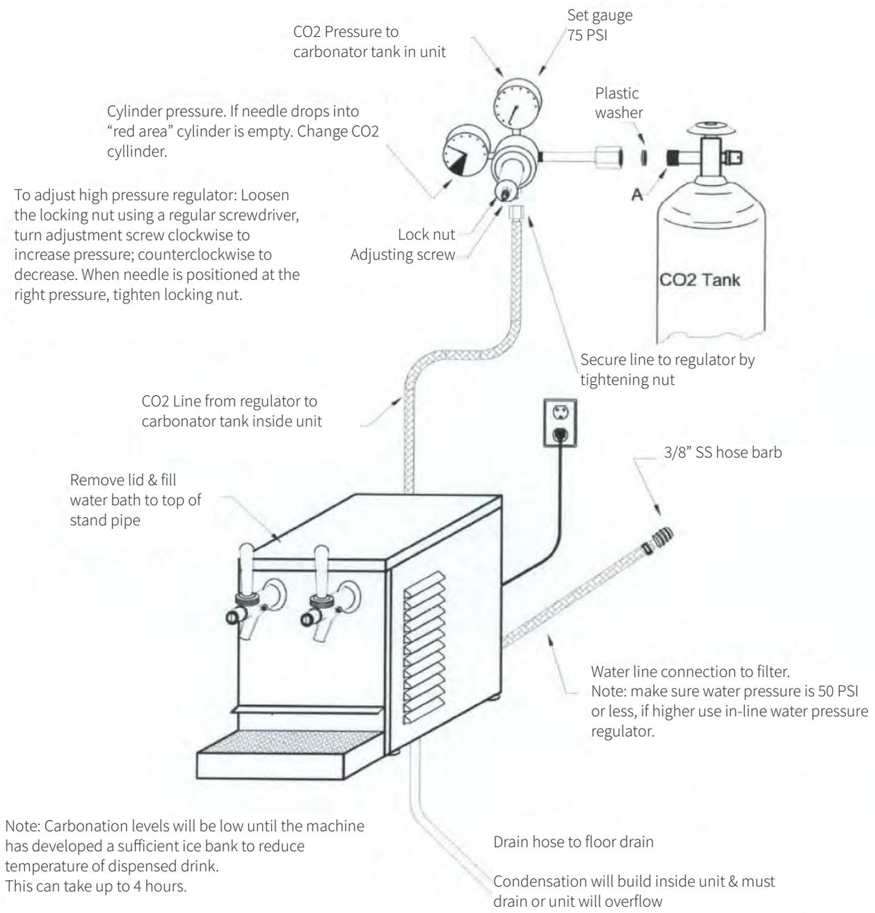
Cylinder pressure. If needle drops into "red area" cylinder is empty. Change CO2 cylinder.
